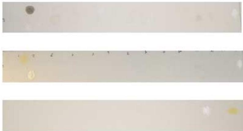
*Figure 3* shows three clear resin products with decreasing effects of the purple stain from the top sample to the bottom sample. All test conditions and timing were identical for the three flooring materials. It is the differences in resin quality with respect to chemical resistance that is responsible for the variations in the performance shown.
