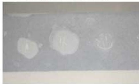
Film softening has an immediate effect on flooring performance. Softened floors will "cut" with heavy-wheeled traffic and quickly erode to the substrate. The softening can initially occur as a surface effect only or as a result of absorption from film swelling. Softening can be seen in Figure 6 as evidenced by the scratches on the surface of the gray resin.
