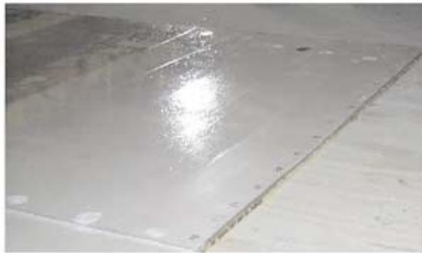
Total film destruction can be seen in *Figure 7* in the spots that appear white. The white appearance is a result of total erosion of the seal coat exposing the white quartz granules in the flooring sample. The two chemicals tested here that resulted in total failure were glacial acetic acid and methylene chloride, both reagent grade.
