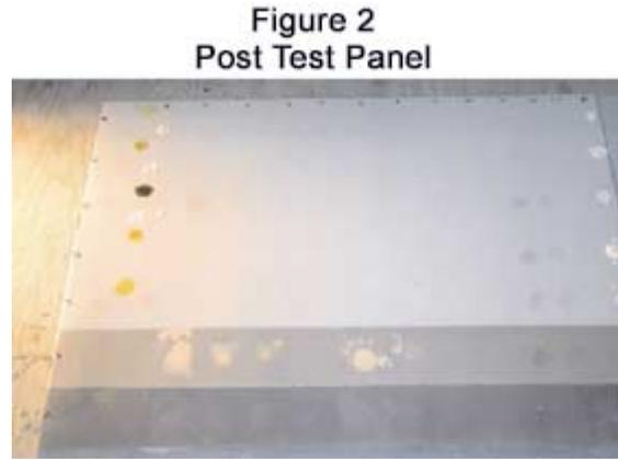
The differences are what we would call remarkable. The most obvious effect in *Figure 2* is what most people generically refer to as "staining". Staining occurs most frequently with no effect to the overall performance of the flooring system. It is a blemish that effects the aesthetic acceptability of a floor only. None the less it is an undesirable consequence. Most of what we see as staining is really discoloration, not staining.
