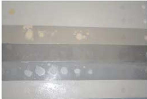
Figure 5 demonstrates film swelling. Film swelling occurs when the resin absorbs the chemical and actually gains volume. Eventually the flooring can have reduced performance properties and deteriorate to the point of failure. Most readings are not as dramatic as the one shown here but are none the less as potentially destructive.
